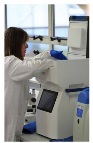
Fig. 4 Via Freeze<sup>™</sup> duo Stirling cycle cooler and operator
